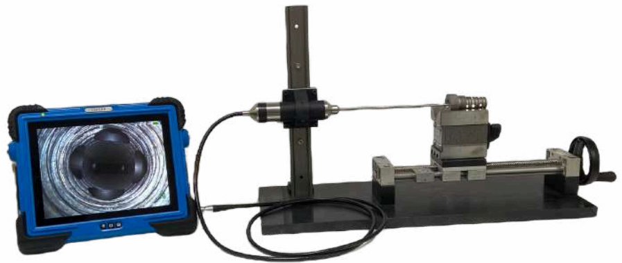
Rigid Borescope and Custom Mechanical Fixture with X, Y, and Z-Axis Movement Control
